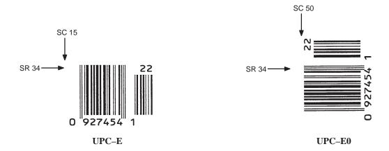
Figure 5-30. Sample UPC-E Bar Codes
